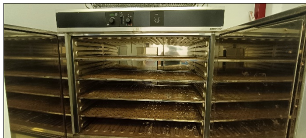
Photo 17. Memmert Be20 oven used for drying the samples.
