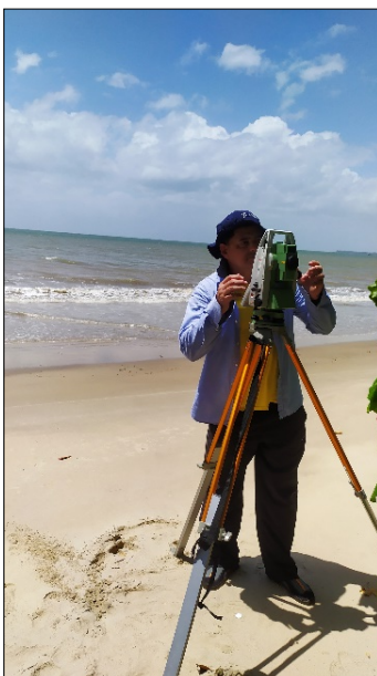
Photos 5-9. Measurement of beach profiles along Bonasse Beach with a Leica TS-09 Plus Total Station.
