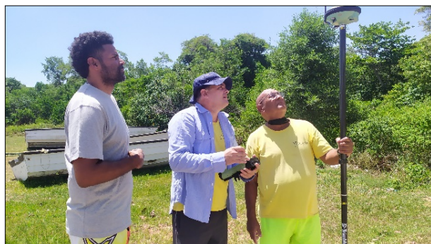
Photos 3 and 4. Establishment of topographic points that serve as heads of the beach profiles for the characterization of the profile morphology.
