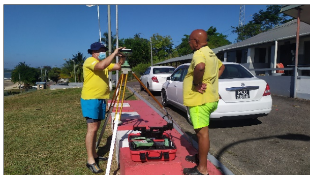
Photos 1 and 2. Installation of the base station at Bonasse Coast Guard facilities. Using GS-14 GNSS Leica in RTK mode.
