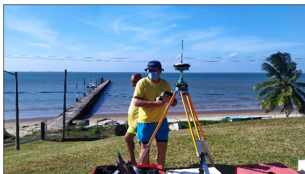
Photos 1 and 2. Installation of the base station at Bonasse Coast Guard facilities. Using GS-14 GNSS Leica in RTK mode.
