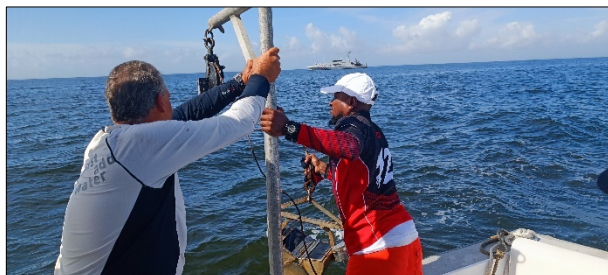
Photos 63 and 64. Collection of sediment samples with using a sampler and winch.
