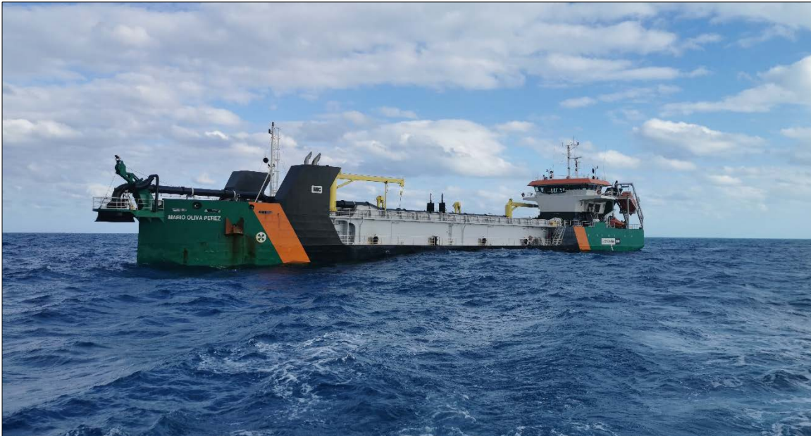
Photo 71. Example of a trailing suction hopper dredger with ideal characteristics for the execution of the project. (Mario Oliva Pérez Dredger, Empresa Constructora de Obras Marítimas, Cuba)
