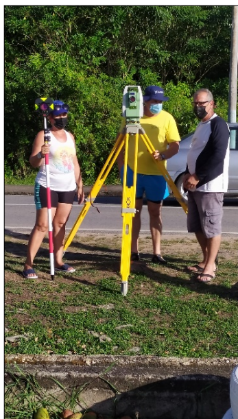
Photos 5-9. Measurement of beach profiles along Bonasse Beach with a Leica TS-09 Plus Total Station.
