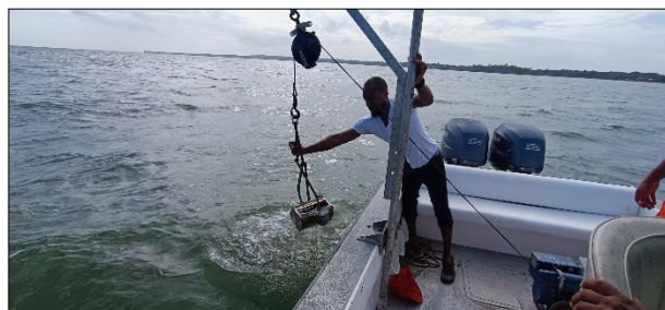
Photos 15 and 16. Use of sampler and winch to collect sand samples at sea.
