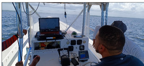
Photos 65 and 66. Execution of the bathymetric survey of the sand borrow area at a scale of 1:15000.
