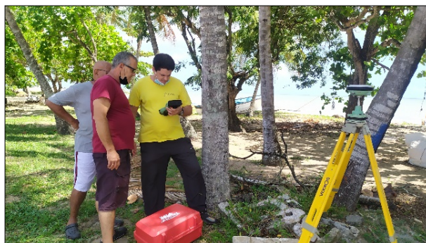
Photos 3 and 4. Establishment of topographic points that serve as heads of the beach profiles for the characterization of the profile morphology.
