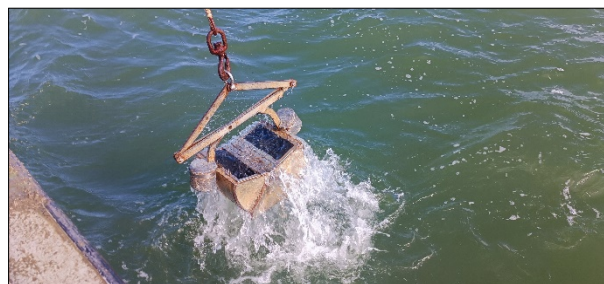
Photos 15 and 16. Use of sampler and winch to collect sand samples at sea.
