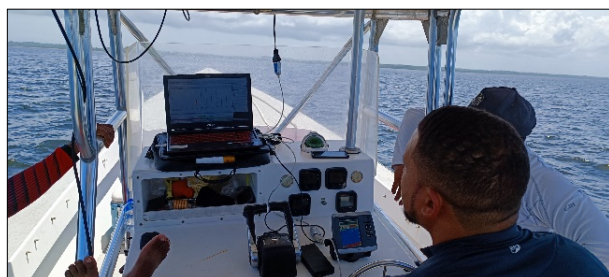
Photos 12 and 13. Execution of the bathymetric survey with the HYPACK MAX 64 software.
