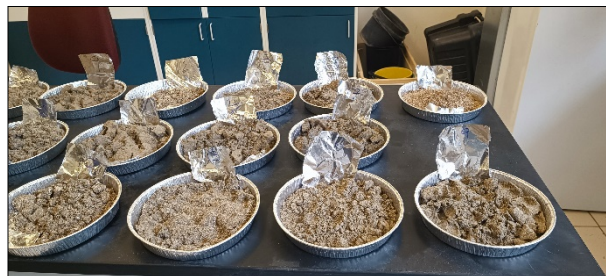
Photo 18. Sand samples dried in the oven for 24 hours.
