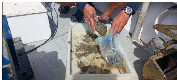
Photos 63 and 64. Collection of sediment samples with using a sampler and winch.
