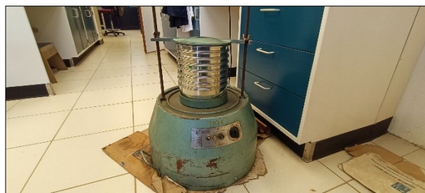
Photo 20. Endecotts Octagon sifter with set of sieves.
