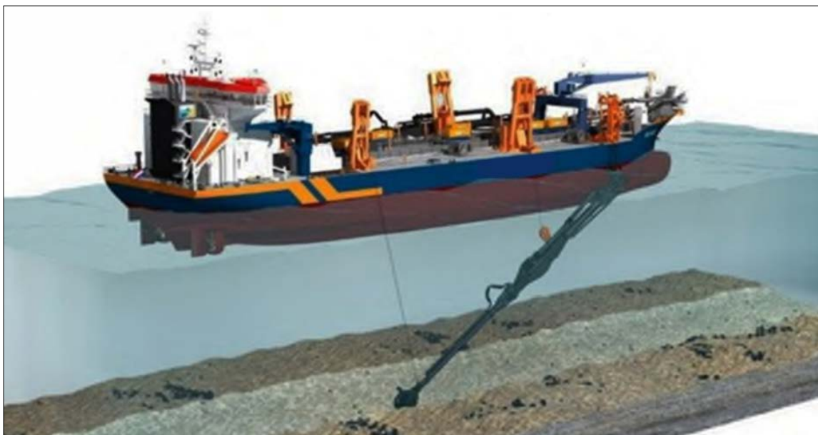
Figure 39. Representation of a trailing suction hopper dredger mining sand with the extended arm.
