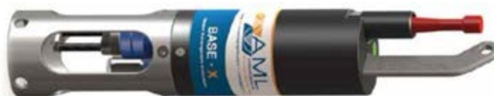
Photo 14. AML sound profiler.
